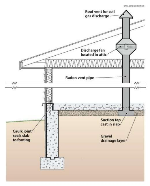
Figure 8. Soil Gas Collection and Discharge Techniques
