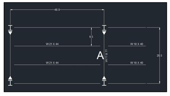
Figure 17: Reduced Beam Designations Influencing Girder A
