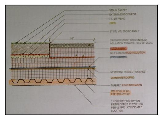
Figure 13: Detailed Actual Extensive Green Roof Assembly
