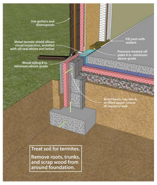
Figure 6. Slab-on-Grade Termite Control Techniques
