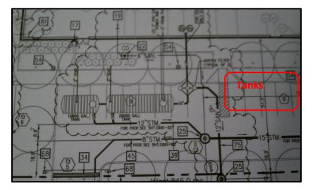
Figure 14: Original Design and Location of Greywater Tanks
