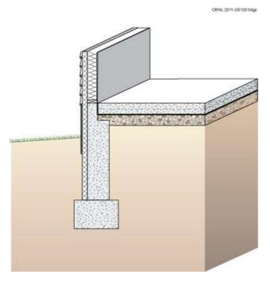
Figure 1. Slab-on-Grade Foundation with Exterior Insulation
