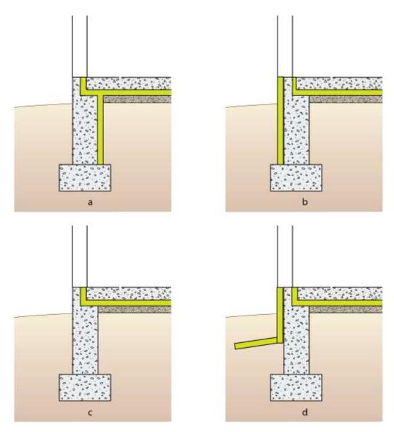
Figure 4. Potential Locations for Slab on Grade Insulation
