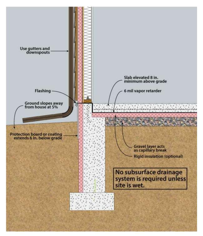
Figure 3. Drainage Techniques for Slab-on-Grade Foundations
