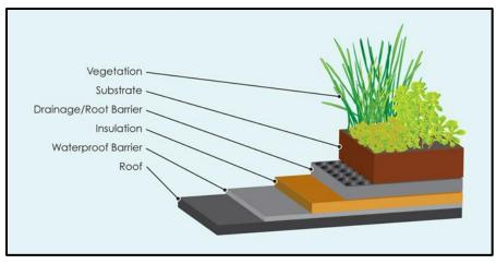
Figure 12: Simplified Extensive Roof Example
