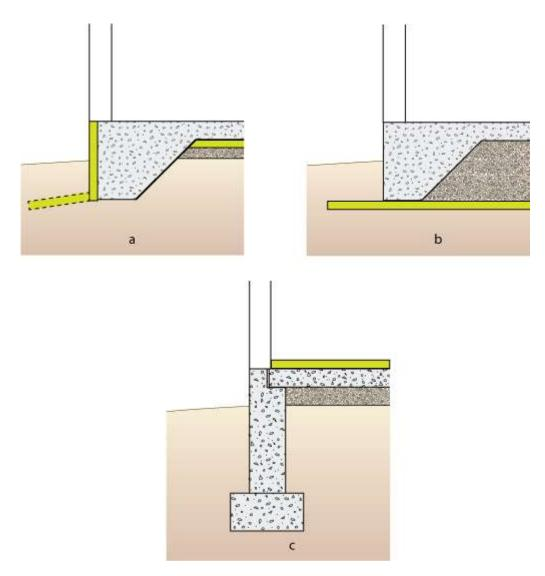
Figure 5. Potential Locations for Slab on Grade Insulation
