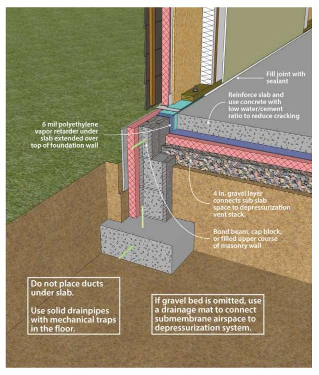
Figure 7. Slab-on-Grade Radon Control Techniques
